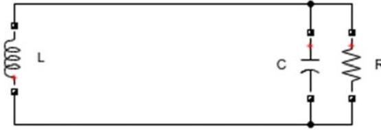
Fig. 3 Switched OFF of Buck-Boost converter
