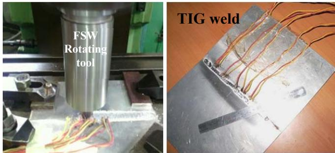
Fig. 1 Experimental set up for thermal characterization in FSW and TIG welds
