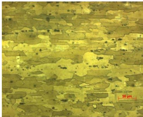
Fig. 7 (a) Microstructure of BM in FSW weld
