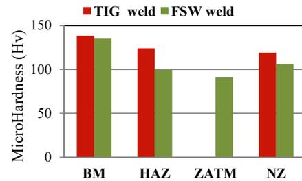
Fig. 5 Microhardness comparison between TIG and FSW welds
