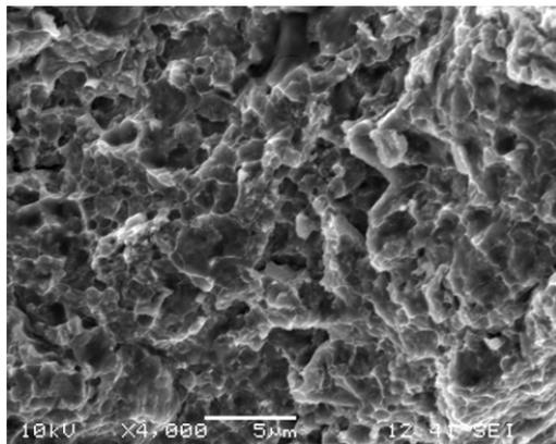
Fig. 6 (b) Fracture surface in FSW tensile tested specimen
