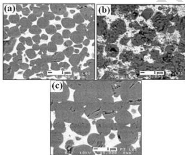
diameter of approximately 2 μm (Table 4) surrounded by the metallic binder. This microstructure contrasts with that of sample  $S_{01}$  (Fig. (4b)), in which the TiC particles are characterized by an intense cracking. The application of load throughout the whole process generates a highly disturbed structure, thus making the TE/HP procedure inefficient.
