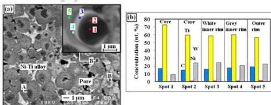
The formation of the core-rim structure seems to inhibit the coarsening of the ceramic particles. These particles had two different appearances (labeled as A and B in Fig. (7a)). The A-type particles had a core-rim structure, in which the core again consists of mixed carbide
