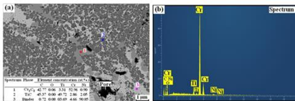
spot spectrum 1) and was associated with the presence of Cr<sub>3</sub>C<sub>2</sub> carbide. Remember that this phase was identified in the XRD pattern (Fig. 2). EDS analysis confirmed that the metal binder consisted mainly of Ni with low contents of Cr and Ti, which were dissolved in the transient liquid phase formed during the thermal explosion process (spot 3). In this cermet, the core-rim structure was not observed in agreement with the literature results.
