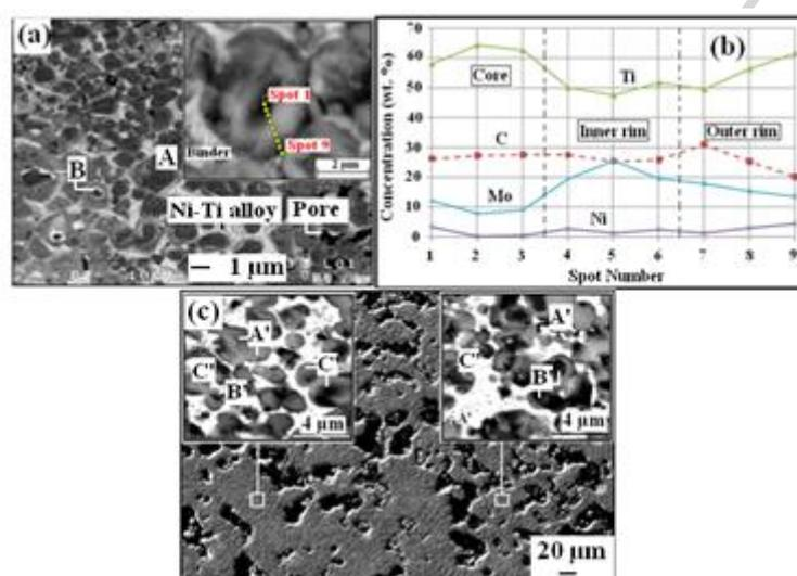
Note that the core, which is the undissolved original particle, is also a mixed (Ti, Mo)C carbide that confirms the formation of this solid solution during the thermal explosion synthesis.
