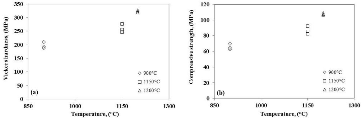
**FIGURE 3.** Mechanical properties using Vickers microhardness for synthesized HAp by calcinations at 900°C and 1200°C and compared to sintered at 1150°C; (a) Hardness, (b) Compressive strength.
