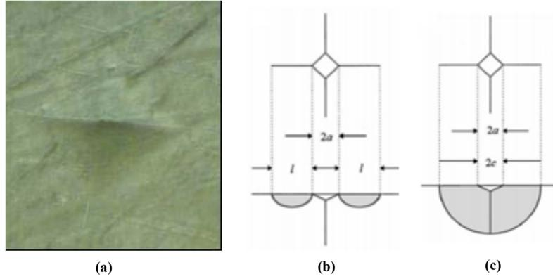
**FIGURE 2.** Cracks obtained by Vickers indentation: (a) Four cracks at the ends, (b) crack under the Palmqvist imprint or "P type", (c) Half penny crack or "M type" imprint [13].
