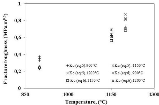
**FIGURE 4.** Fracture toughness for synthesized HAp by calcinations at 900°C and 1200°C and compared to sintered at 1150°C.
