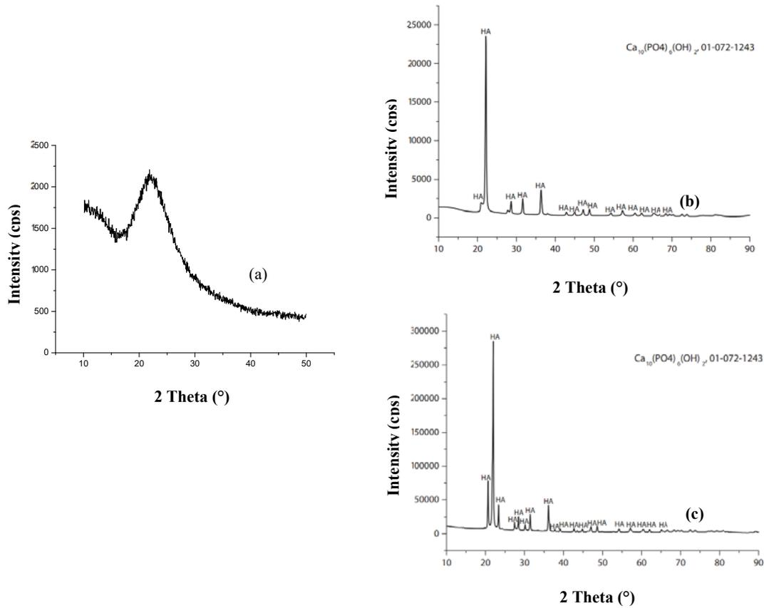
**FIGURE 1.** X-ray diffraction thermograms of stoichiometric HAP:
