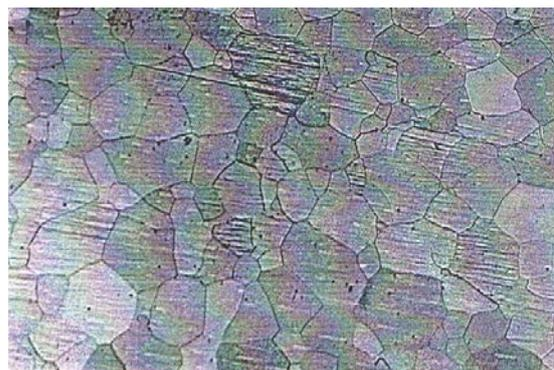
Figure 1. Optical micrograph of original structure of ferritic stainless steel type 409 supplied for the present work. X50
