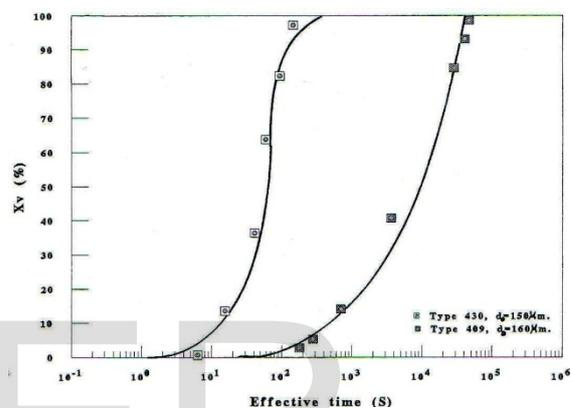
Figure 6. Isothermal recrystallisation kinetics of ferritic stainless steel type 430 and 409, deformed at an effective strain of 0,58 and at a temperature of  $870^{\circ}\text{C}$ .
