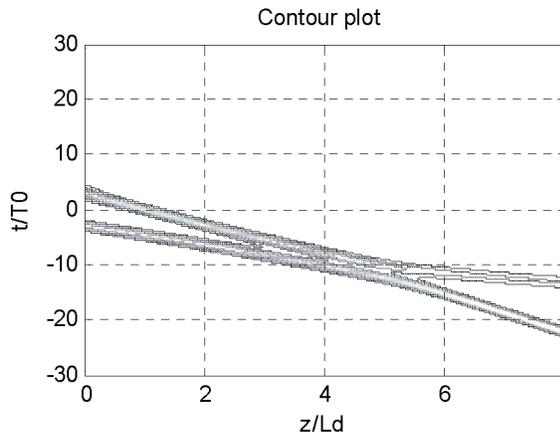
**FIGURE 2** Contour plot showing the collision between two solitons in the same channel.
