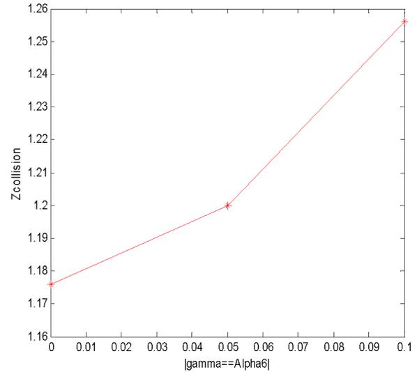
**FIGURE 3** Influence of the quintic nonlinearity on the collision length between neighboring solitons in the same channel.
