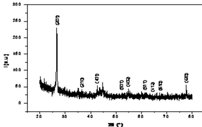
Figure 1: XRD patterns of  $MnO_2$  thin films on to graphite substrate
