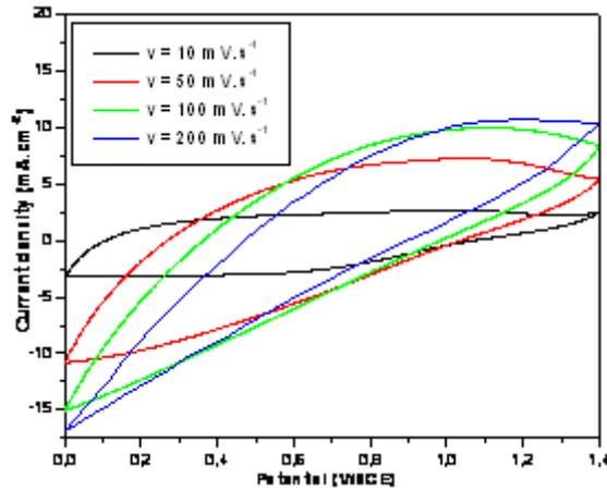
Figure 3: Cyclic voltammetry for MnO<sub>2</sub> thin films
