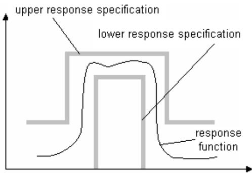
Figure 2: filter specification
