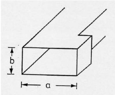
Figure 1: Waveguide inductive discontinuity.
