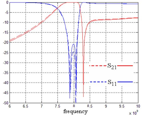
Figure 8: Superposition of our results (broken line) and HFSS response.
