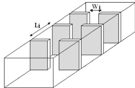
Figure 4: waveguide filter and geometrical unknown factors.
