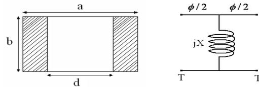
Figure 3: Cross sectional view and inductive iris equivalent circuit
