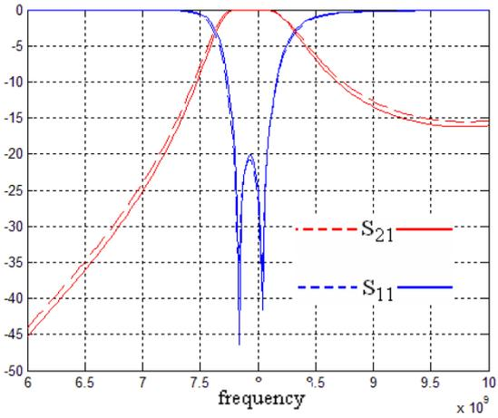
Figure 6: Superposition of our results (broken line) and HFSS response.
