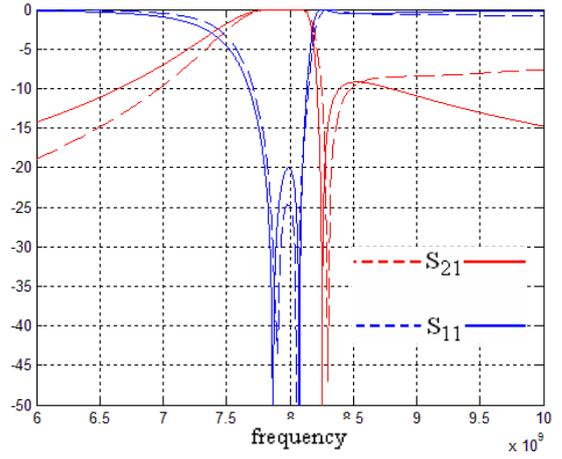
Figure 7: Superposition of waveguide filter (broken line) and equivalent circuit response
