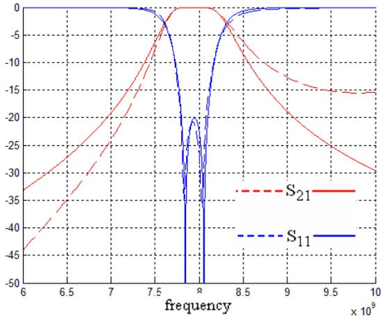
Figure 5: Superposition of waveguide filter (broken line) and equivalent circuit response
