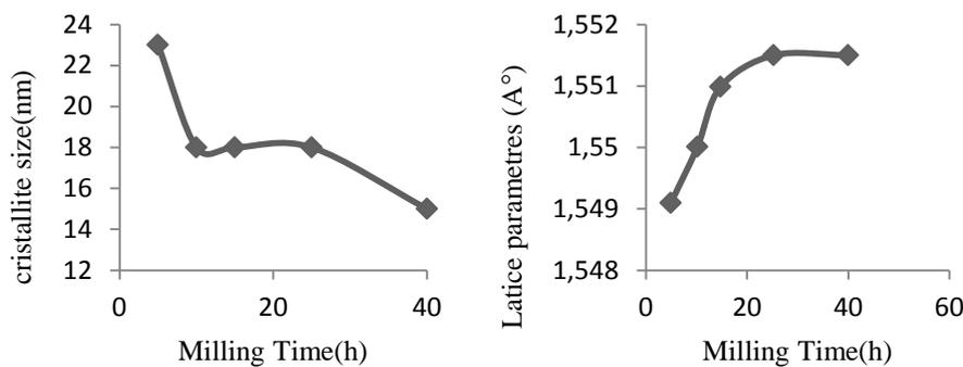
Fig.6: Evolution of crystallite size and lattice parameter during milling
