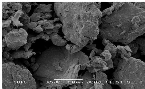
Fig.2: initial stage of mechanical alloying (Fe-Co after 5 h of milling).
