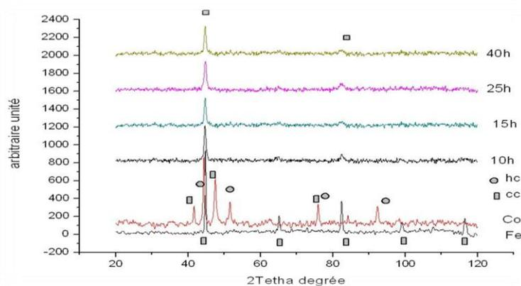
Fig.5: X-Ray Diffraction evolution of Fe-Co alloy during milling.
