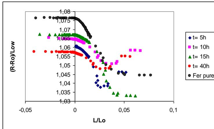
Figure (9): Eddy current measurement (Impedance diagram)
