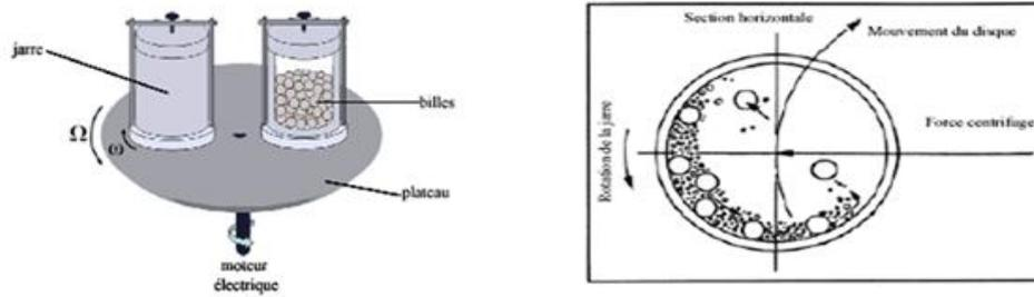
Fig.1: Mechanical milling
