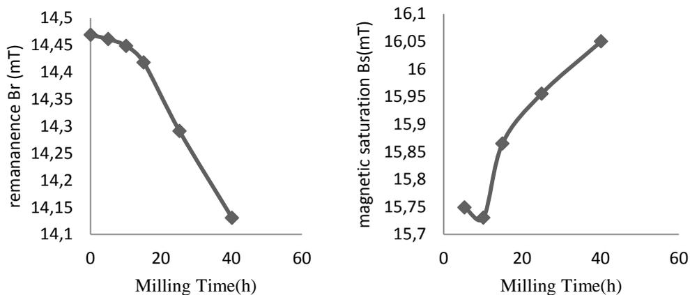
Fig.8:  $B_r$  and  $B_s$  evolution during milling.
