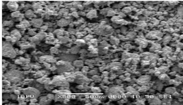
Fig.4: final stage de of mechanical alloying (Fe-Co after 15h of milling).
