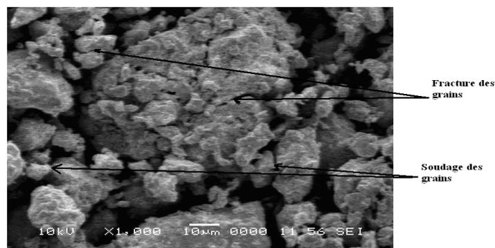
Fig.3: intermediate stage of mechanical alloying (Fe-Co after 10 h of milling).
