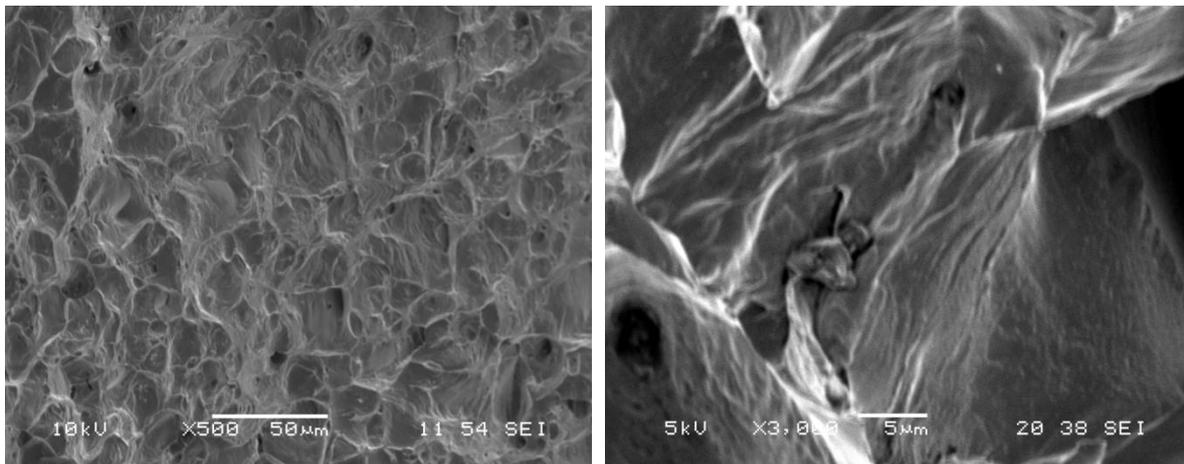
Fig.11: Rupture fractography of samples (1080 and 1120°C) after restoring at 1080°C.
