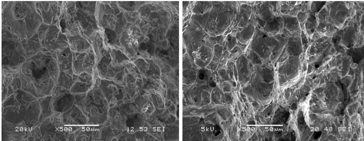
Fig.6: Rupture fractography of samples (1080 and 1120°C) after ageing at 850°C.
