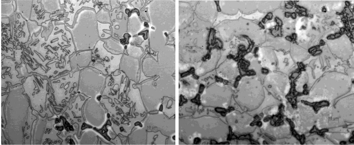
Fig.7: Optical micrographs obtained from DSS 2205 annealed at 1120°C and aged at 850°C for: (a) 30 min, (b) 60 min, (c) 90 min, (d) 120 min.
