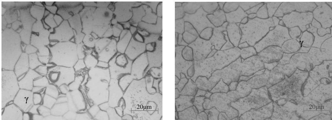
Fig.3: Optical micrographs of the specimens aged at 850 °C after being solution-treated at 1080 °C and 1120 °C.
