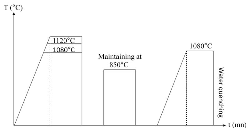
Fig.1. Diagram sequences of performed heat treatments.
