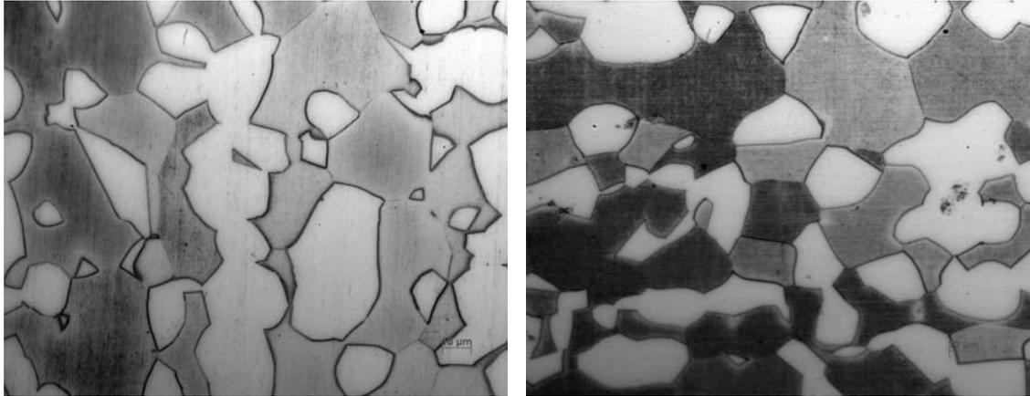
Fig.8: Optical micrographs obtained from DSS 2205 annealed at 1080°C for 60min. Respectively: (a) 1080/60-850/60. (b) 1080/60-850/120.
