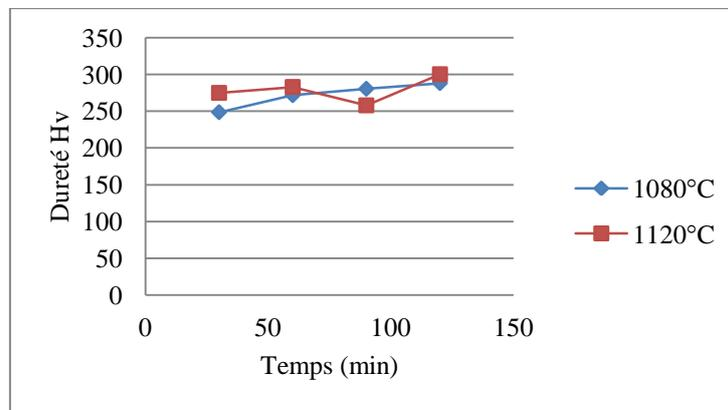
Fig. 5: Effect of aging times at 850°C on Vickers hardness.
