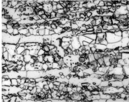
Fig.2: Microstructure of sample in the as received condition, consisting of austenite (light etched) and ferrite (dark etched).
