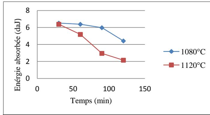
Fig. 4: Effect of aging times on absorbed energy of DSS 2205 at 850°C.
