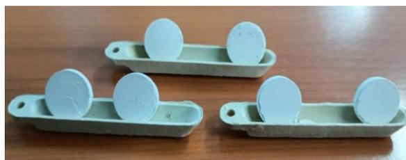
Figure 2 Pellets before sintering.
