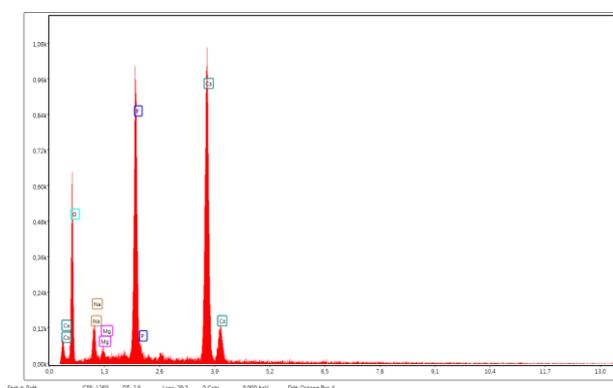
Figure 5 EDS analyses of the pellet surface after 5 days of immersion in SBF.
