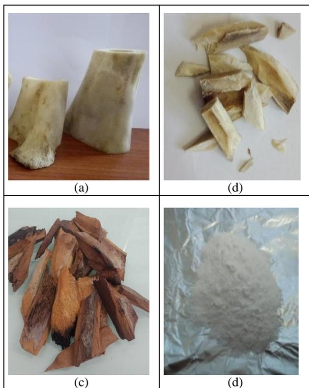
Figure 1 Powder preparation cycle, a) Bovine bones, b) Small pieces of bone, c) Bones heated at 400°C, d) Bones calcined at 900°C.
