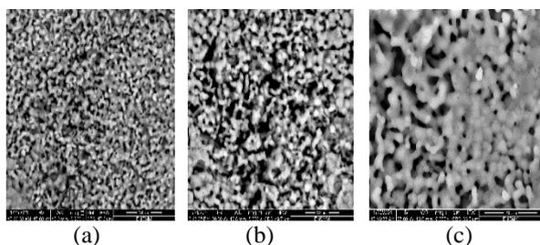
Figure 4 SEM morphologies of the pellet surface after immersion in SBF, a) 1 day, b) 5 days, c) 14 days.
