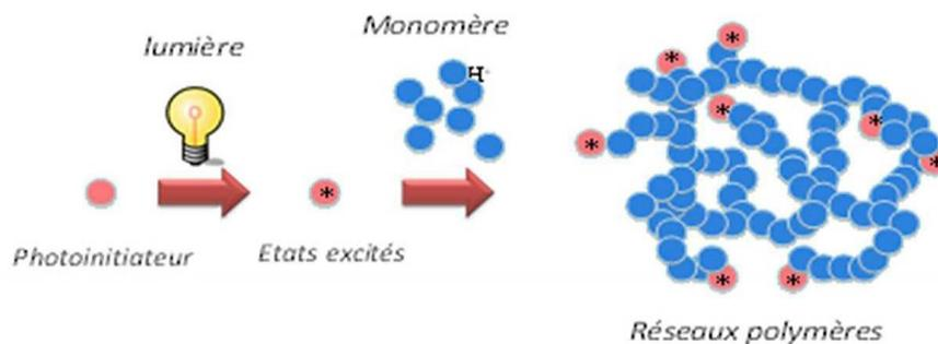
**Figure 1:** Schematic diagram of the light curing process.
