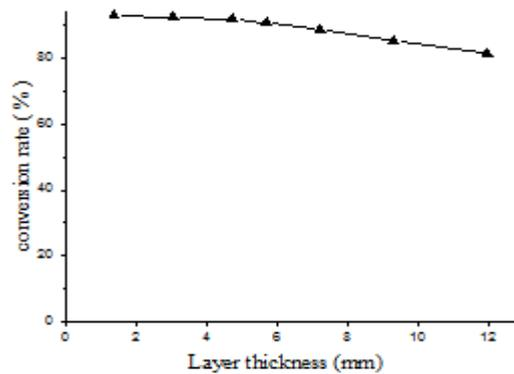
**Figure 5:** Conversion rate as a function of layer thickness.
