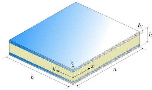
**Figure 1.** Geometry and coordinate system of sandwich composite plate.
