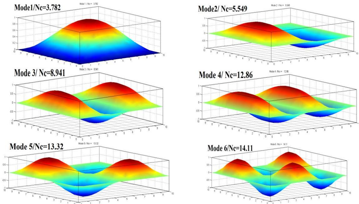
Figure 5. Six first buckling modes for an uniaxial buckling load of a simply supported sandwich square plate from the developed element
