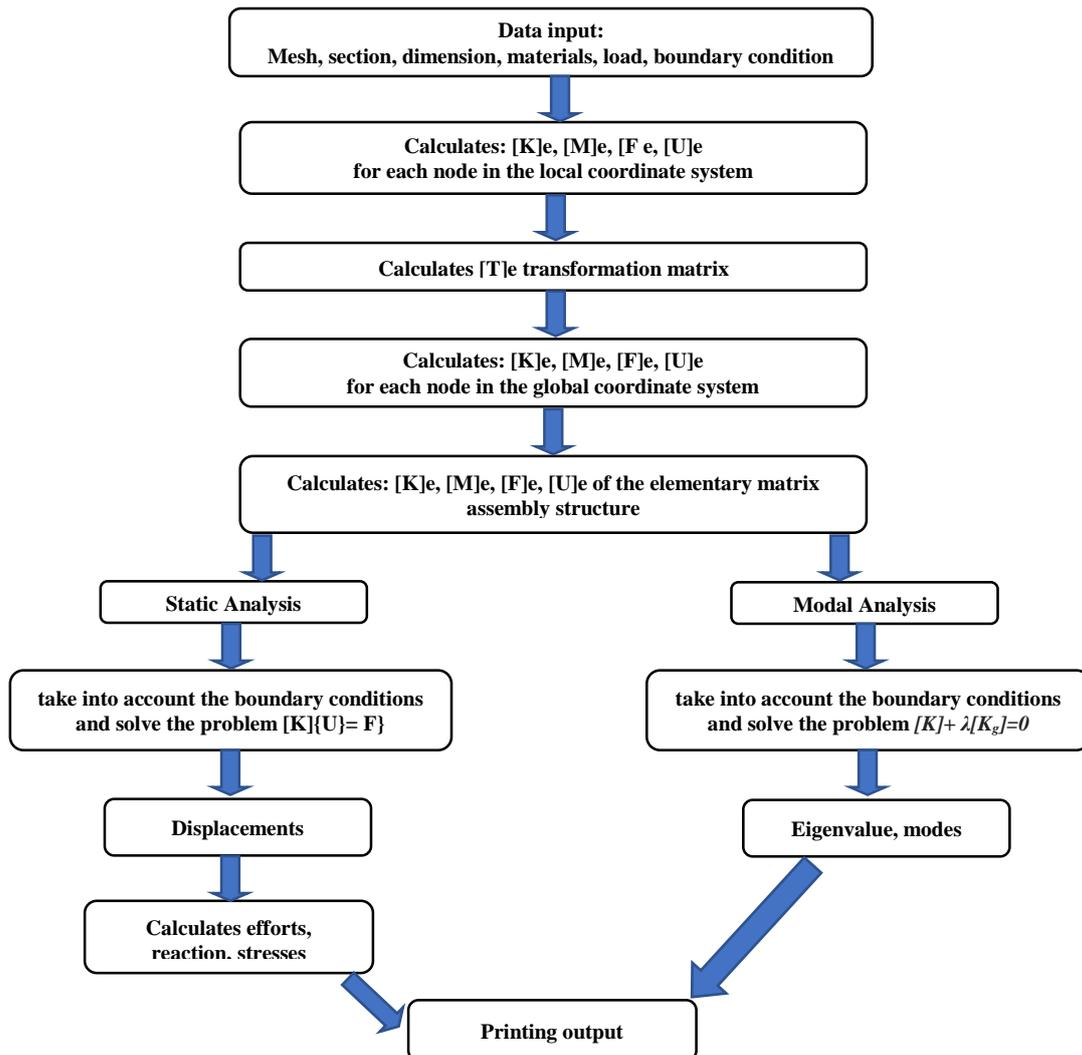
**Figure 3.** Program of the developed numerical finite element model.
