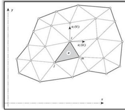
**Figure 2.** Finite element meshing description of a solid
