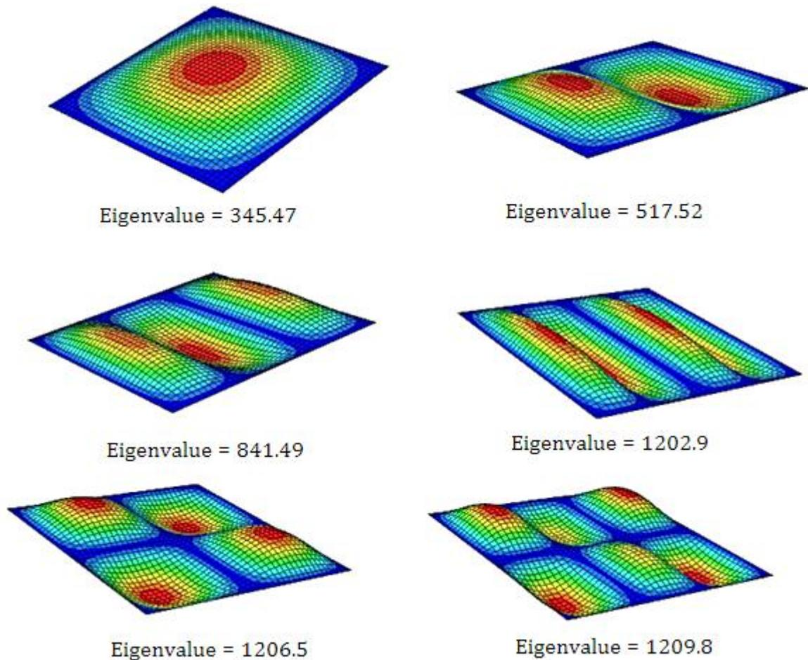
**Figure 6.** Six first buckling modes for an uniaxial buckling load of a simply supported sandwich square plate from the Abaqus element S4R
