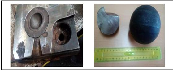
Figure 1: Used steel ball forging die and forged ball
