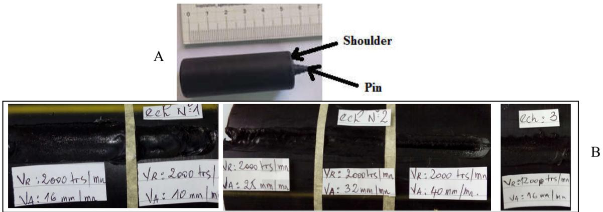
Fig. 2 .A The welding tool, B pehd welded samples
