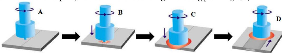
Fig .1. The four stages of the FSW process: (A) The tool is rotated, (B) penetrations, (C) shoulder is brought into contact with the surface of the parts to be assembled, and (D) Welding phase.
