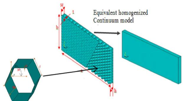
Fig.1 Equivalent parameters of a honeycomb sandwich plate.
