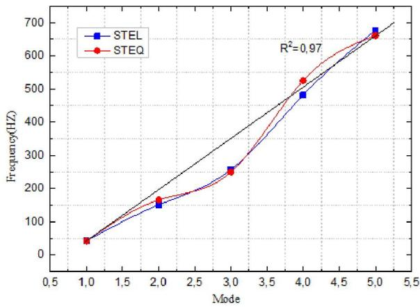
Fig.2 Comparison between FEA and equivalent methods for large frequency.
