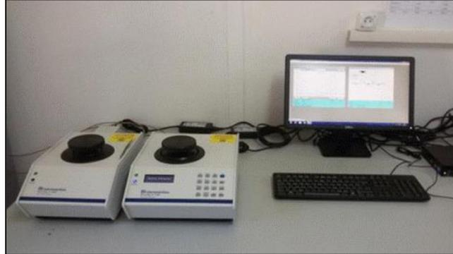
**Figure 3.** Micromeritics AccuPyc II 1340 Gas Pycnometer.
