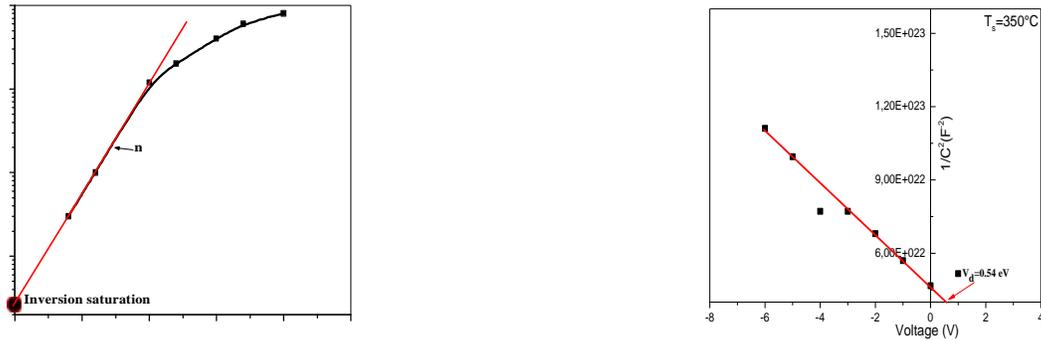
**FIGURE 5.** (h) : The corresponding logarithmic scale in current with forward bias condition of ZnS/SnS heterojunction at room temperature of SnS film grow at 350°C.
