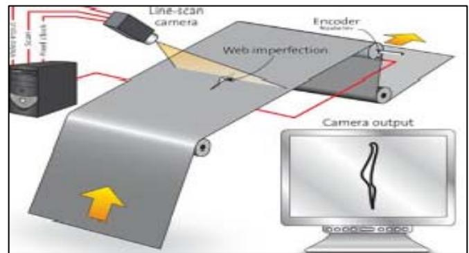
Fig. 1. Detection system of steel strip defects based on machine vision.
