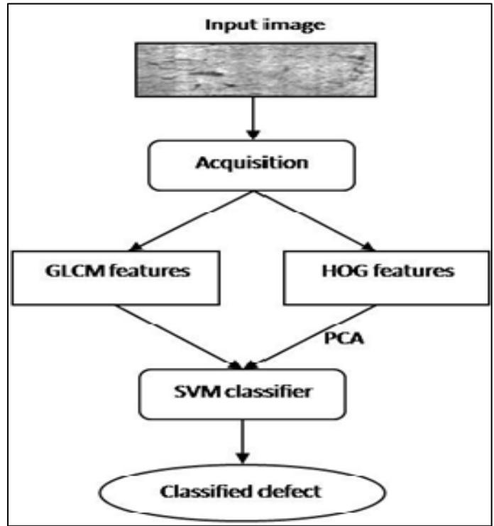
Fig. 2. Block diagram of the proposed system.
