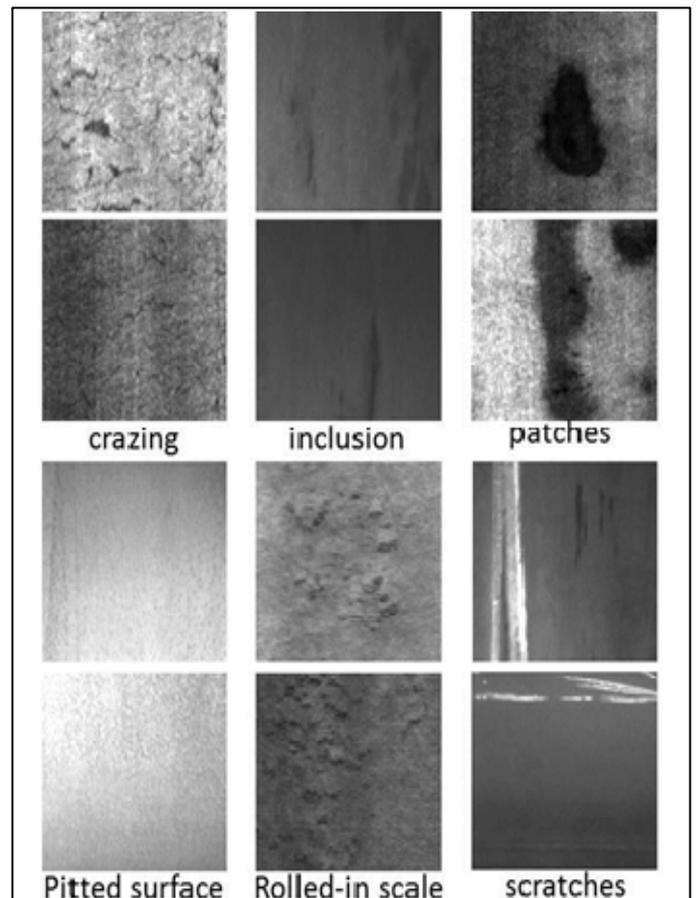
Fig. 3. Samples images of six classes of typical surface defects.
