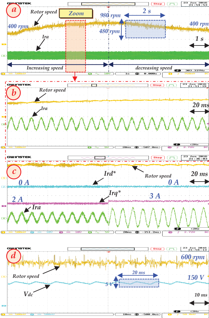
Fig. 7 (a) & (b): Steady and transient states respectively of increasing and decreasing rotor speed and rotor current, (c) variation of the rotor reference direct current, (d) transient and steady states of bus voltage.
