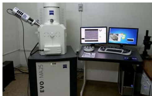
Figure 2. Electron scanning microscope of type Zeiss EVO MA25.
