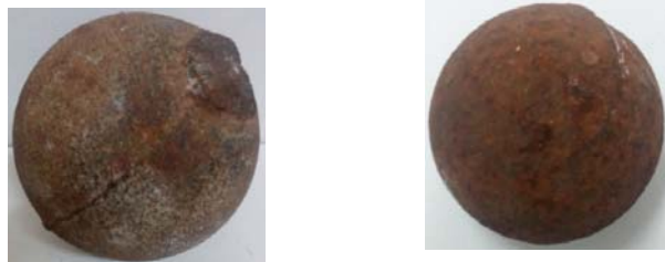
Figure 1. A) ball obtained by molding, B) ball obtained by forging
