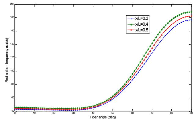
Fig. 4. Effect of angle of fiber on fundamental natural frequency of the cracked composite beam for different crack location  $x/L=0.3, 0.4, 0.6$
