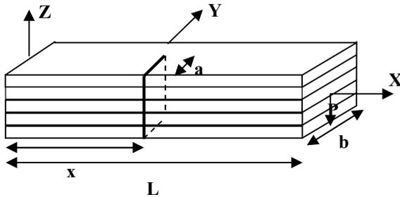
Fig 1. Geometry of cracked composite beam
