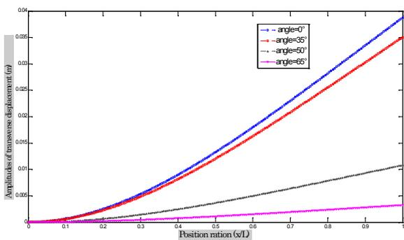
Fig. 6. Amplitudes of transverse displacement of composite beam for different fiber angle .
