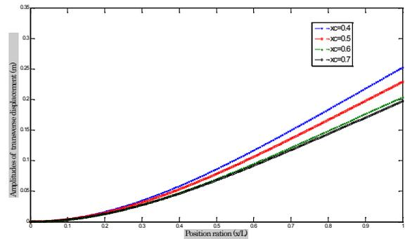
Fig. 8. Effect of crack position on the amplitudes of transverse displacement of composite beam
