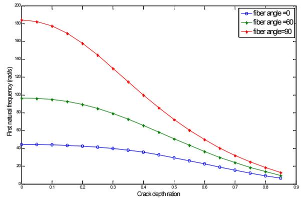
Fig. 3 Effect of crack depth on fundamental natural frequency of the cracked composite beam for different angle of fiber
