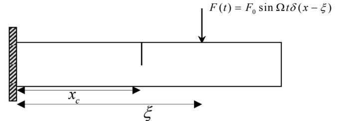
Fig.2. Cracked composite beam subjected to concentrated harmonic force.
