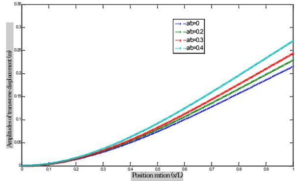
Fig. 7. Effect of crack depth on the amplitudes of transverse displacement of composite beam
