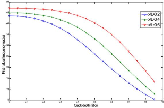
Fig. 5. Effect of crack depth on fundamental natural frequency of the cracked composite beam for different crack location ratio  $x/L=0.2, 0.4, 0.6$
