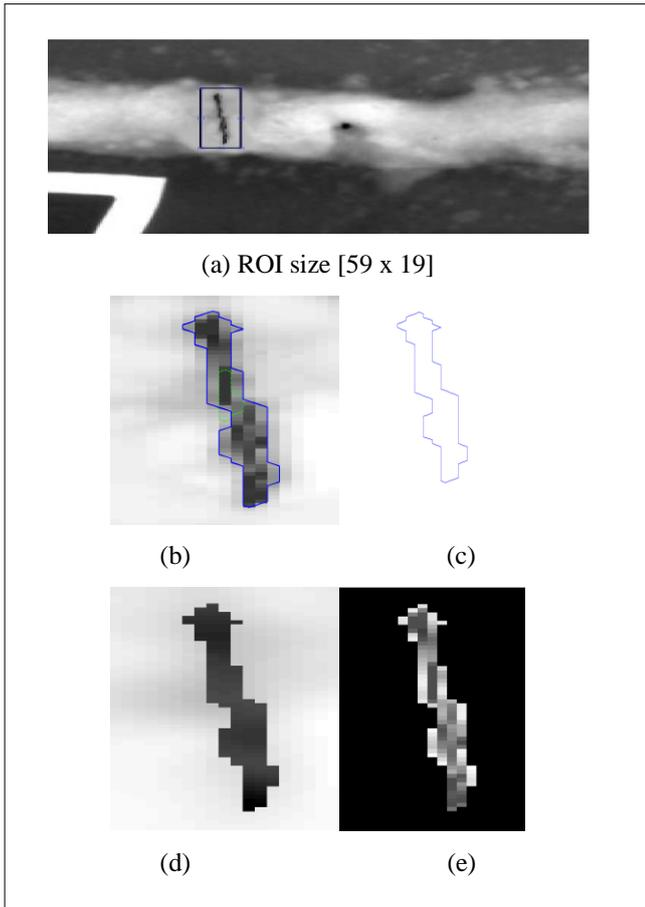
Fig. 4. Weld defect segmentation and restoration from the second rough radiographic image: (a) Defined ROI in rough weld radiographic image, (b) ROI image with initial contour (dashed green line) and final contour (solid blue line), (c) Edge defect, (d) restored weld defect, (e) Weld defect with its initial grey scale.  $\sigma=3$ , iteration=1900, CPE time=12.78s.
