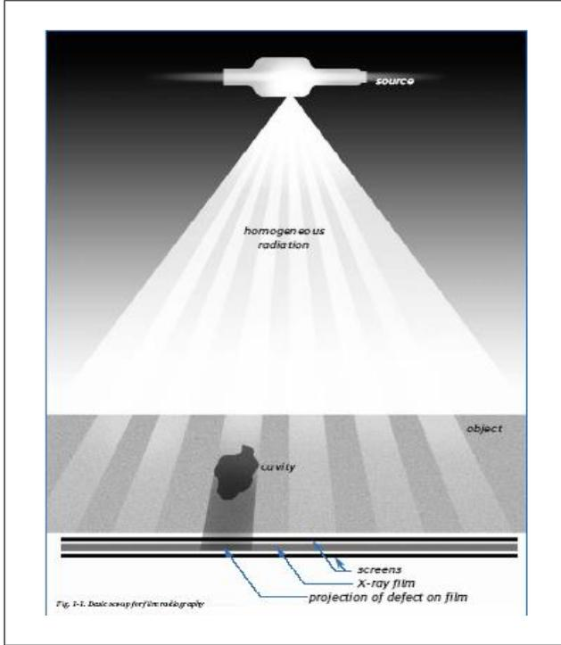
Fig. 1. Industrial radiography image forming technique [26].
