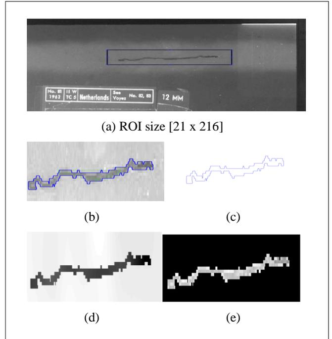
Fig. 5. Weld defect segmentation and restoration from rough radiographic image: (a) Defined ROI in rough weld radiographic image, (b) ROI image with initial contour (dashed green line) and final contour (solid blue line), (c) Edge defect, (d) restored weld defect, (e) Weld defect with its initial grey scale.  $\sigma=3$ , iteration=1000, CPE time=2.82 s.
