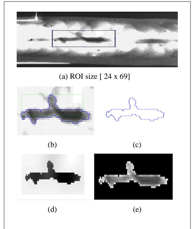
Fig. 3. Weld defect segmentation and restoration from rough radiographic image: (a) Defined ROI in rough weld radiographic image, (b) ROI image with initial contour (dashed green line) and final contour (solid blue line), (c) Edge defect, (d) restored weld defect, (e) Weld defect with its initial grey scale.  $\sigma = 5$ ,  $iteration = 250$ ,  $CPE\ time = 2.82\ s$ .
