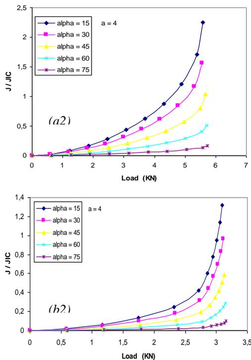
Fig. 11. Curve J- Applied load for (a/w=0,25), (a2) BM, (b2) WM
