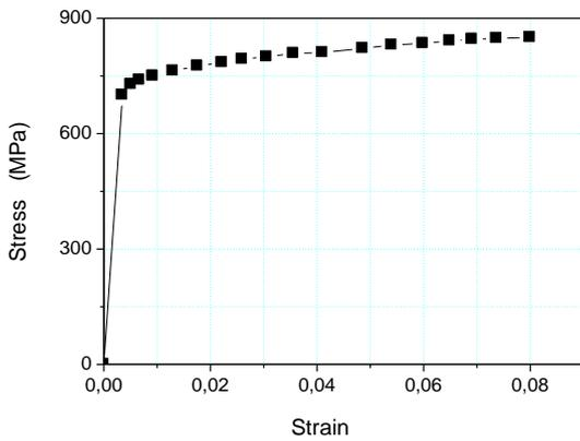
Fig. 2. Uniaxial stress–strain curve of the steel at room temperature [17].
