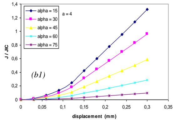
Fig. 10. Curve J-Displacement for (a/w=0,25), (a1) BM, (b1) WM
