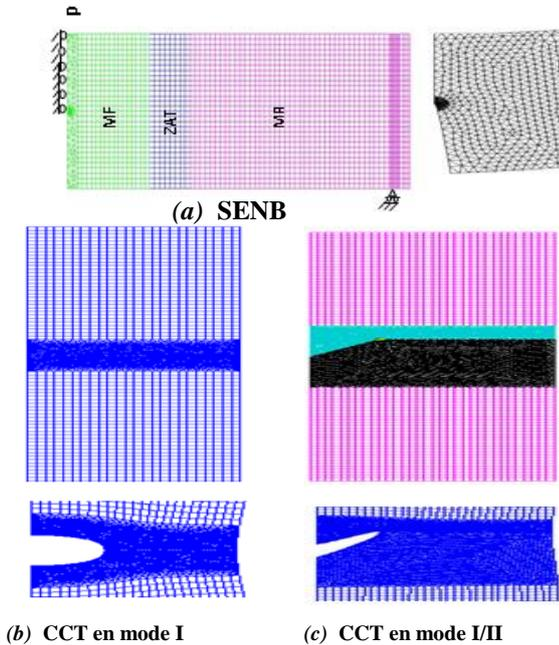
Fig. 3. Finite element discretisation scheme: global view and zoomed view near the crack tip
