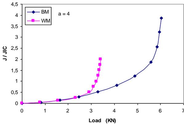
Fig. 7. Curve J- Applied load for (a/w=0,25)
