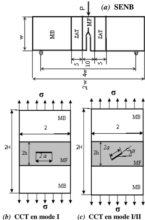
Fig. 1. Schematic models analyzed: (a) TPCB (SENB); (b) CCP1 and (c) CCP2
