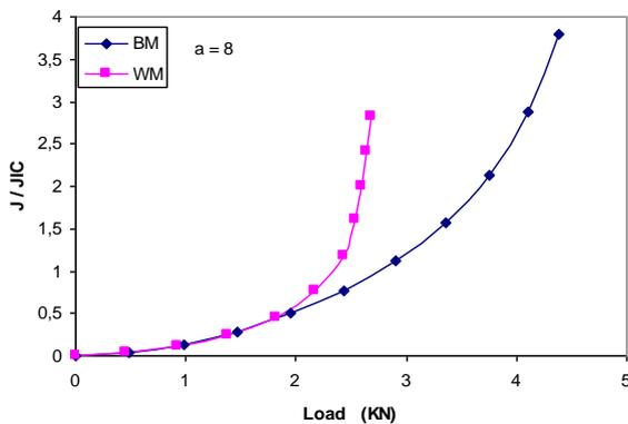
Fig. 9. Curve J- Applied load for (a/w=0,5)
