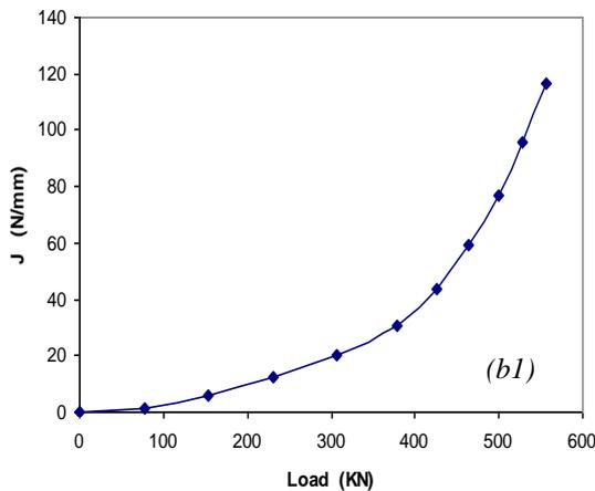
Fig. 5. Curve J- Applied load for (a/w=0,5)
