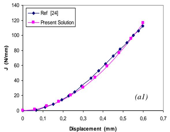
Fig. 4. Curve J-Displacement for (a/w=0,5)
